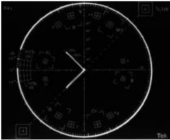
Figure 18. The 1781R polar SCH phase display showing a 10 degree error.
