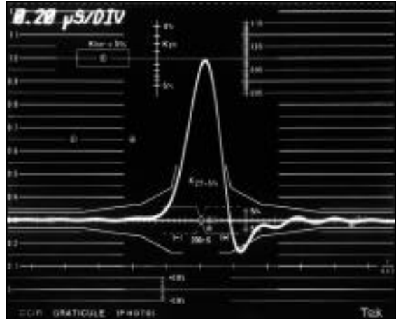
Figure 57. A 2T pulse properly positioned for a K_{2T} measurement. This signal has a K_{2T} distortion of slightly more than 5%.
