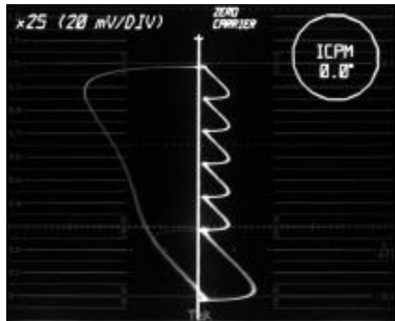
Figure 102. 1781R ICPM display with no distortion present.
