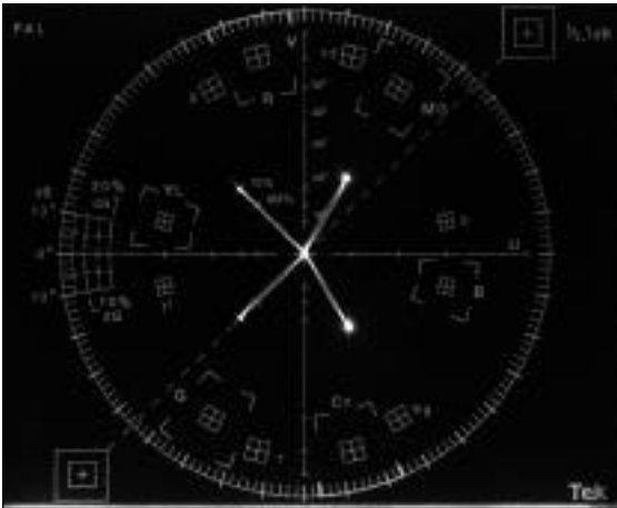
Figure 63. Vector display of the TG2000 phase-alternate modulated ramp.
